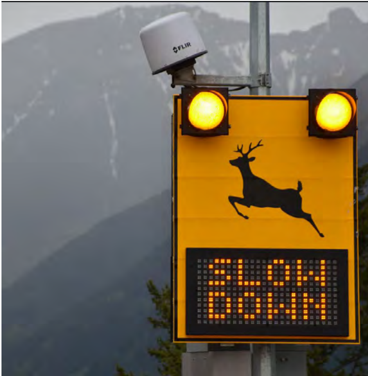
Animal Detection System on Highway 3, Alberta
